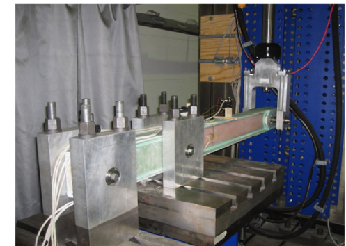
Fatigue tests on Henkel beam at Fraunhofer IWES
